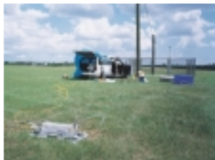
The Tekran Model 2537A inside the monitoring van is being used by Oak Ridge National Laboratories to monitor mercury emissions from ground covering a landfill in Florida. A Teflon flux chamber is visible in the foreground.
